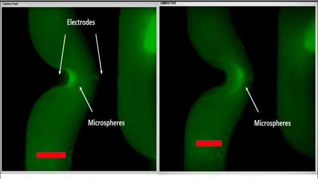
Images illustrate repositioning of microsphere cluster after changing the electricity frequency. The repositioning shown here took place in 40 milliseconds. The position of the cluster and the rate at which the cluster moves is used to determine presence and quantity of the target molecule bound to the microspheres. Red bar = 50 microns.
